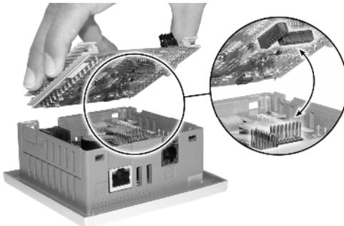
1. Gently replace the board. Make certain that the pins fit correctly into their matching receptacle. Do not force the board into place; doing so may damage the controller.
