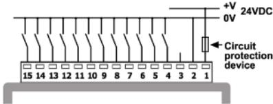
HSC input wiring, npn (sink)
