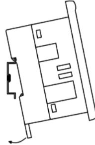
2. When properly mounted, the controller is squarely situated on the DIN-rail as shown in the figure to the right.
