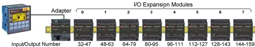
The module is supplied with a set of labels – select the label appropriate to the position of the module. For more information, refer to the *Configuring I/O Expansion Modules* topic in the on-line help of the software supplied with the controller.
